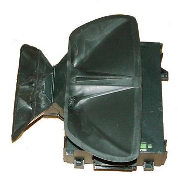
The interior protection sensor is an ultrasound-based (USIS) motion detector which detects all movements inside the vehicle interior and evaluates them using the DWA logic.
